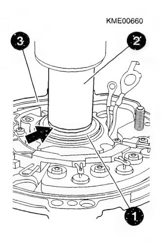
Assembling windingless rotor
